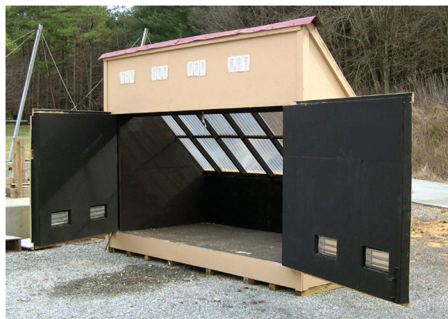
Figure 4—A solar kiln in the United States with rear doors. The drawings at the end of this publication depict a design that incorporates the doors at the front end of the kiln.
