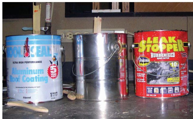
Figure 3—Coatings that can be used to seal the inside walls of the kiln and to coat the ends of sample boards. From left to right: aluminum roof coating, a commercial kiln coating, and rubberized roofing sealer.
