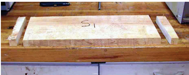
Figure 7—Dimensions and picture of sample board for controlling the drying process.
