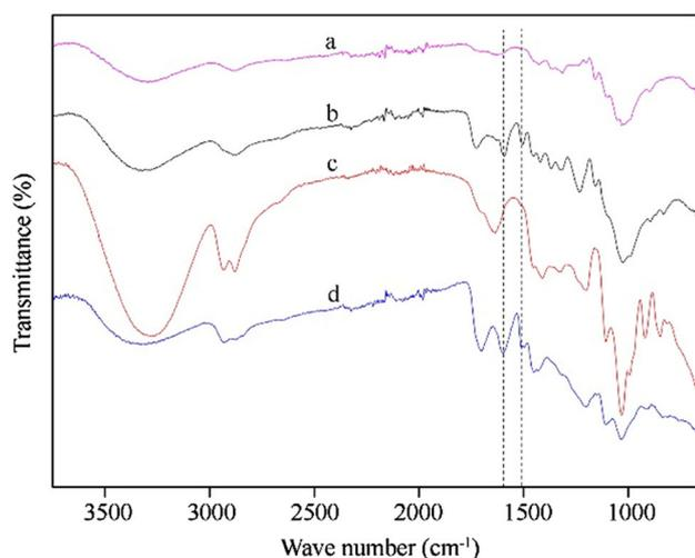
**Fig. 4** FTIR spectra of (a) liquefied residue, (b) raw material, (c) water soluble content, (d) precipitate content. Liquefaction conditions: solvent glycerol/methanol of 2/1, microwave power of 300 W, sulfuric acid of 1.75 % (w%), solvent/bamboo of 4/1, temperature of 150 °C, and time of 7 min
