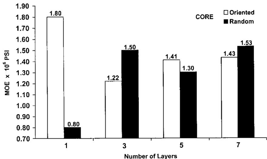
Figure 2. — MOE of panels fabricated with different layers as affected by core construction.
