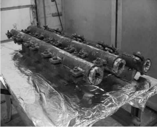
FIG. 4. Small-scale wood composite poles being pressed in steel molds.
