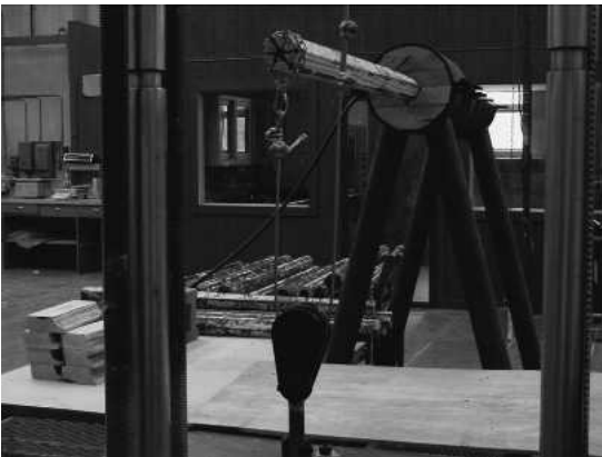
FIG. 5. A small-scale composite pole being tested in a RIEHLE machine.
