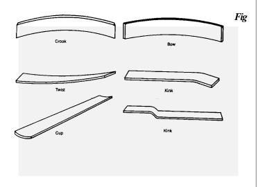
*Figure 5.* Drying defects that can occur in improperly seasoned lumber.
