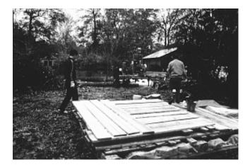
*Figure 6b.* A poor stacking job with no stickers between boards. There is little ventilation under or inside the pile. Lumber piled in this fashion may lead to warp, check, stain and decay.
