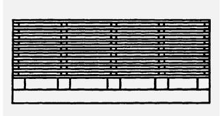
*Figure 13.* A properly stacked pile of lumber has stickers of equal thickness that are vertically aligned. The normal distance between stickers and braces is 18-24 inches.
