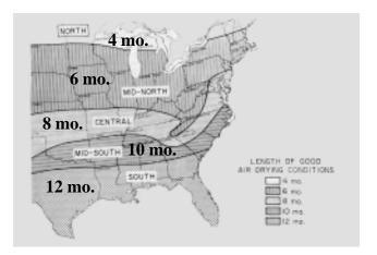
*Figure 4.* Air-drying map for the Eastern United States. Source: McMillen and Wengert (1978).
