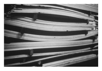
*Figure 12.* This lumber has experienced severe bow because these stickers and braces have been placed too far apart.
