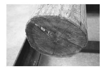
*Figure 15.* Checks and separation occurred in unprotected ends of this hardwood log during storage in the log yard at the sawmill before milling. End checks can be reduced by end coatings and prompt sawing.
