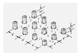
*Figure 7a.* A good foundation is needed for correct stacking and good seasoning. Use treated wood, steel or concrete.
