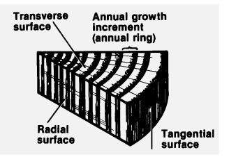
*Figure 2.* The three primary surfaces of wood. Dimensional movement is unique in each of these three planes. (Source: USDA Forest Products Laboratory 1987)
