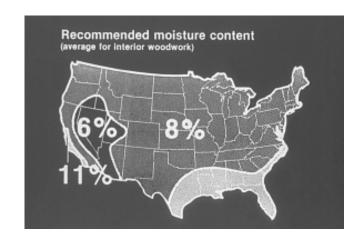
*Figure 3.* The recommended moisture content at the time of installation for interior wood and wood-based products varies throughout the country. Producers should be aware of the recommended moisture content values for wood and wood-based products when selling goods to these areas. Source: Peck (1955).
