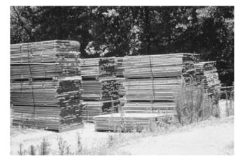
*Figure 6a.* A poor commercial site for seasoning native hardwood. This low-land site has poor air circulation and is subject to flooding. Stacks should be covered.
