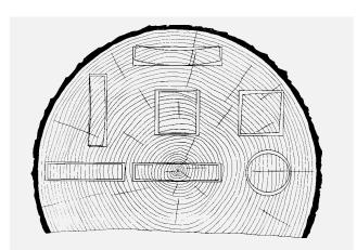
**Figure 1**. Wood shrinkage and distortion of flats, squares and rounds as affected by the pattern and direction of annual growth rings. (Source: USDA Forest Products Laboratory 1987)
