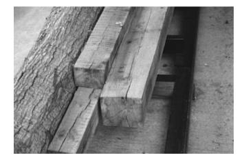
*Figure 16.* End checks in cants caused by rapid drying and sun exposure. End checks that develop in logs will also be present in the lumber that is sawn.
