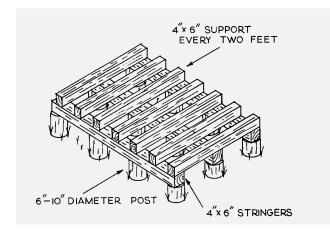
*Figure 7b.* Start the pile by alternate placing of all the shorter lumber inside the layer. Orderly piling and spacing make for good ventilation and even drying. Do not allow lumber ends to hang over more than 6 inches.
