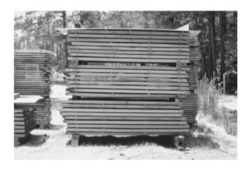
*Figure 9.* Good seasoning practices include a level, welldrained open area that is not subject to flooding. Foundations should hold the lumber at least 15 inches above the ground and a fastened roof or cover to protect wood from rain. Orient stacks to reduce sun exposure and increase air flow, usually north to south stacks.
