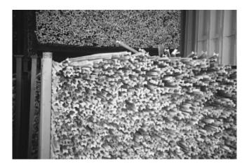
*Figure 8.* A new form of sticker is shaped like a dog bone. These stickers provide maximum ventilation between adjacent lumber, because they are curved and have less surface area in contact with the boards. These stickers will provide better ventilation than traditional stickers and minimize the possible area for the transfer of stain from a sticker to a board (sticker stain). It is always important to keep stickers dry and discard stained or broken stickers immediately.
