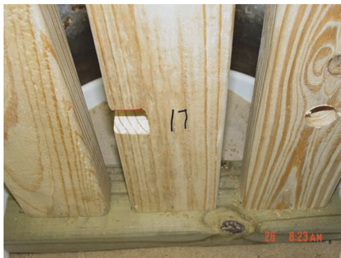
Figure 6. High termite mortality in the sand and sill on the fourth day of the test.
