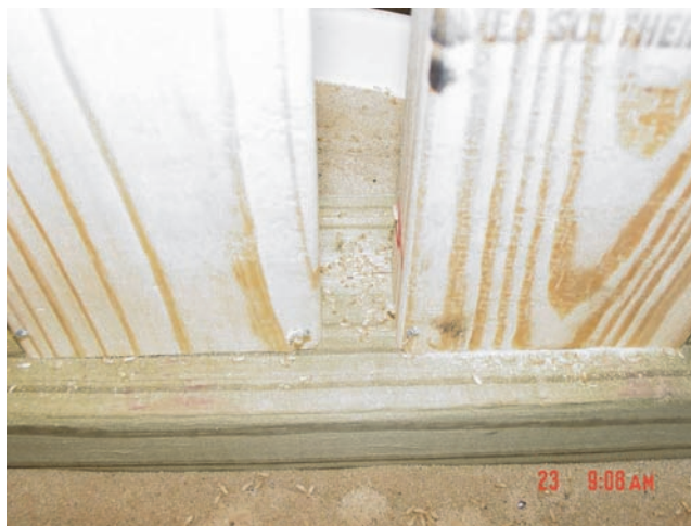
Figure 5. Low termite mortality on a sill plate on day two.
