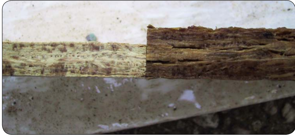
Close-up end view of OSB (left) and wetted OSB (right) that has absorbed water and swelled. (Photo provided by Steve Easley, Steve Easley & Associates, Inc.)
