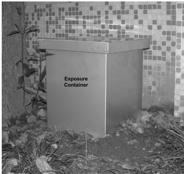
Fig. 1. Rectangular stainless steel exposure container (300 × 300 × 450-mm high, 20-liter volume) containing pyrethroid-, solvent-, and nontreated specimens with P. radiata sapwood strips and blocks (Fig. 2) in a C. formosanus -infested site, Guangzhou, China.
