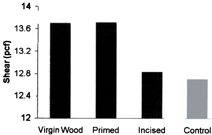
Fig. 5. Surface treatment effects on the bonding shear of laminates made from decommissioned CCA-treated utility poles.
