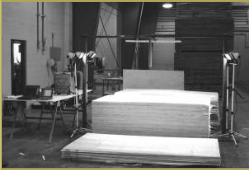
Figure 7. — Process monitoring for the assessment of veneer in the manufacture of plywood using a portable NIR spectrometer.
