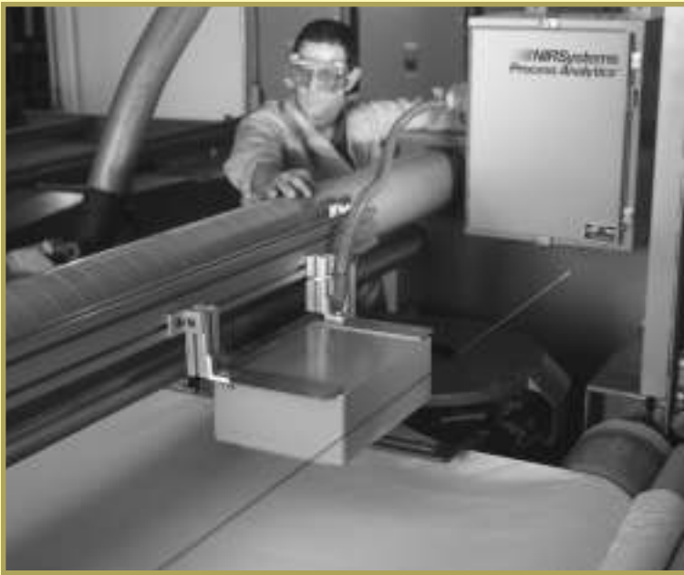
Figure 6. — Integrated NIR instrument for online process monitoring. Photo courtesy of Foss NIRSystems.
