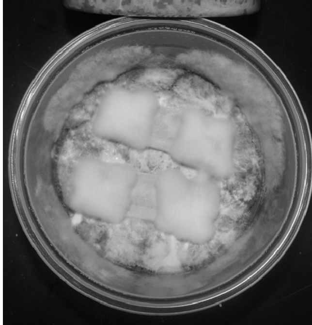
Figure 1. Photo is a depiction of one container holding 4 exposed wafers of a particular retention covered by mycelium of P. placenta .
