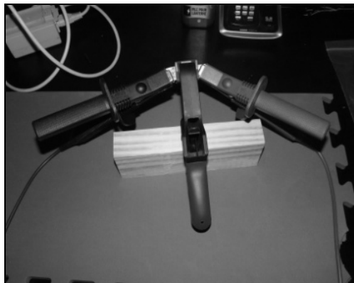
Figure 5. Solid copper plates were adhered to a non-conductive plastic clamp to which roughly five pounds of force was applied securing each wafer in-between the copper plates so that the copper plate was larger than the wafer sample to ensure that the entire wafer was exposed to the electrical current.
