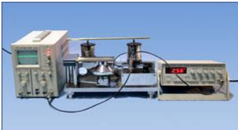
Fig. 1. DY-D99 dynamic multifunctional measuring instrument for determining Young's modulus
